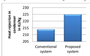
due to the helical shape of the condenser. The heat rejection was increased from 214KJ/Kg to 225KJ/Kg.
